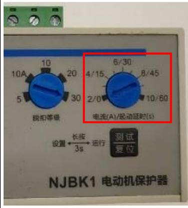
The image shows the front panel of the NJBK1-80 motor protector after improvement. The right-hand rotary knob now has a scale that includes '6/30', '4/15', and '8/45' in addition to the previous values, indicating the addition of a start delay function. The text 'NJBK1 电动机保护器' is visible at the bottom. | 增加启动延时功能标识            |
