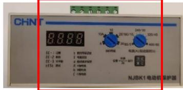
The image shows the front panel of the NJBK1-400 motor protector after improvement. The digital display and rotary knobs are now positioned higher and more centrally on the panel, making the appearance more uniform with the other models. The text 'NJBK1 电动机保护器' is visible at the bottom.                 | 显示屏和旋钮位置居中靠拢，系列外观更加统一 |
