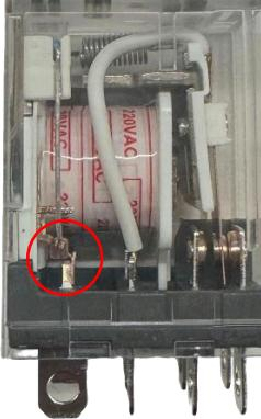
A photograph of the same relay component after the manufacturing process change, showing a single red circle highlighting a small metal clip or fastener that has replaced the soldered connection.          |
